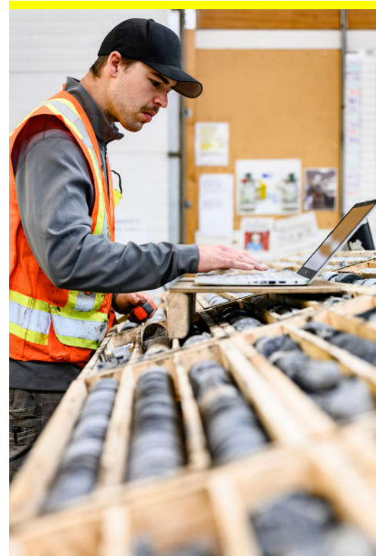
At Keno Hill, a worker analyzes core samples from exploration efforts in the mine.
