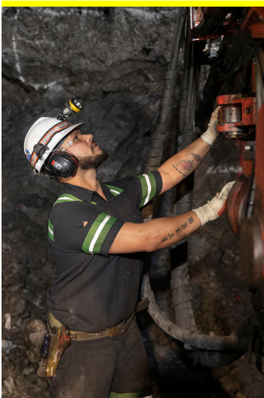
Utilizing a mechanized rock bolter, a miner anchors bolts in a stope wall to support excavation at Greens Creek.
