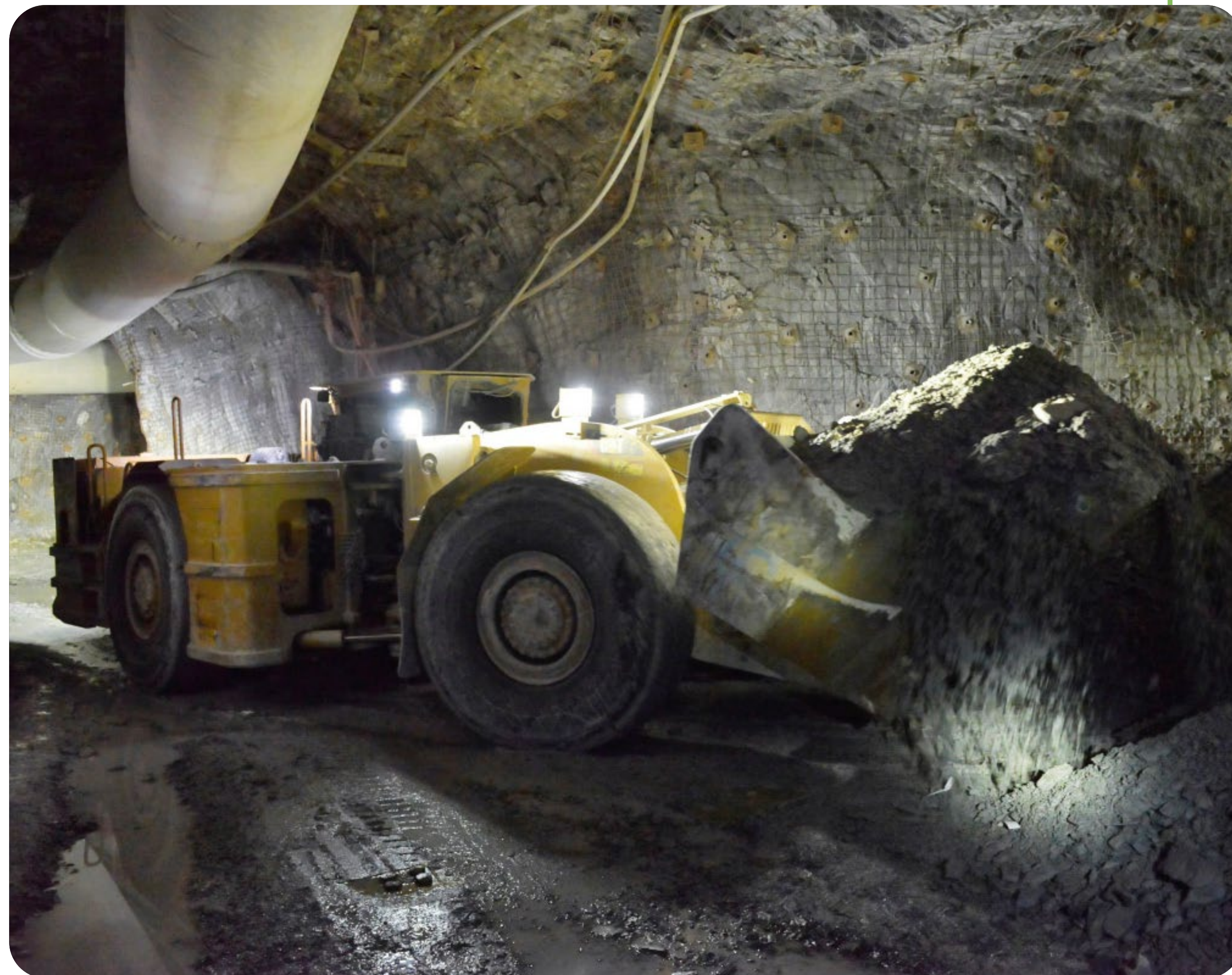
Underground loader at Lucky Friday
