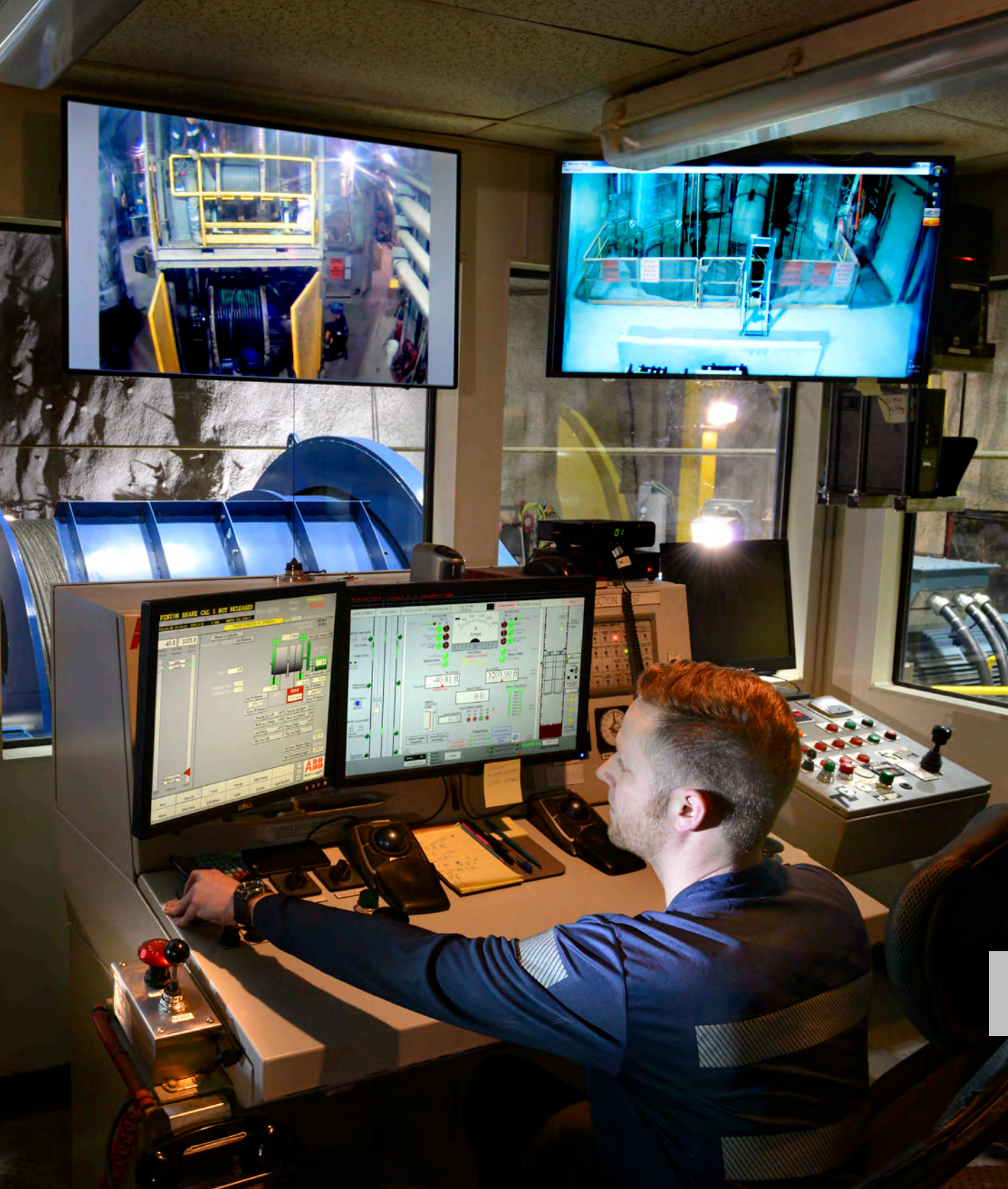
The new #4 Shaft hoist control room at the 4900 level of the Lucky Friday mine.
